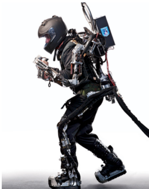
Figure 4: Sarcos Exoskeleton, adapted from Michael, (2009)
