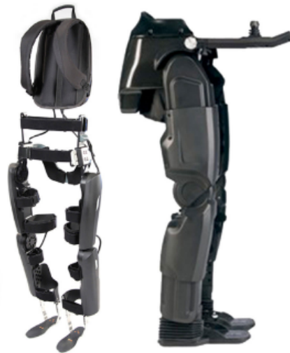
Figure 5: The ReWalk exoskeleton, adapted from Michael, (2009)
